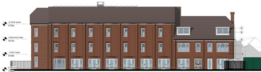
Proposed East Elevation 1 : 100
